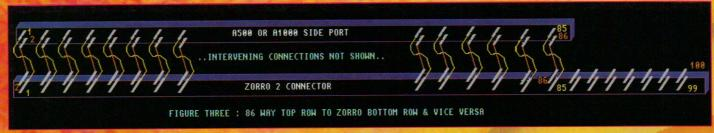
There is a whole lot of soldering to be done here. The top row of pins need on the 86-way connector need to be connected to the bottom row of pins on the 100-way and vice-versa. It would be a good idea to mark some numbers on the ends before you start.
