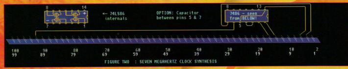
The logic chip connections should be made to the pins of the DIP socket. It is quite simple to connect the socket to the connectors, but make sure you put the chip in the right way round!
