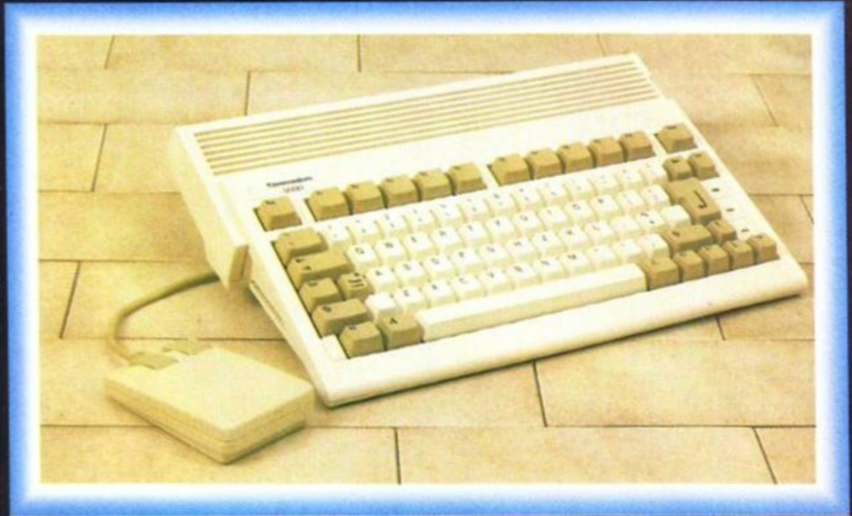
TWO MODELS: A600 FD Single 3.5" 880Kb. Floppy Drive A600 HD Single 3.5" 880Kb. Floppy Drive with internal 20Mb. Hard Disk Drive.
