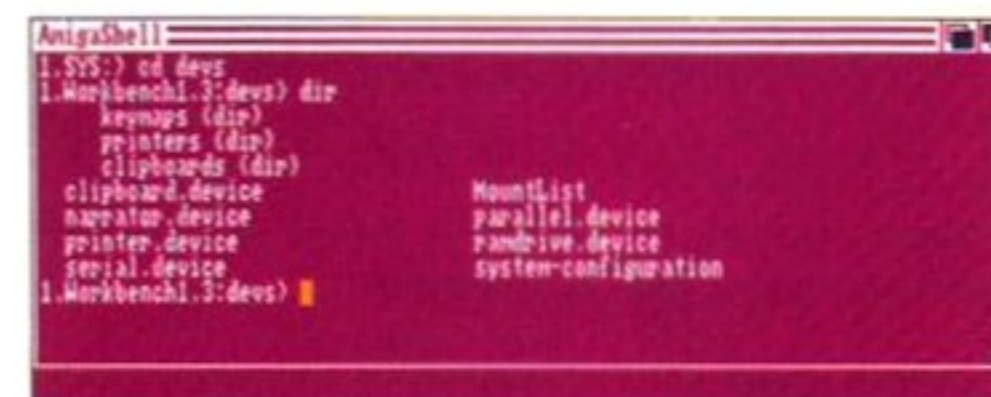
We can get the system-configuration file we want from the Workbench disk's own devs directory. This means that your self-booting disk will have the same Preferences setups as your Workbench: like the gaudy maroon colour, in my case!
