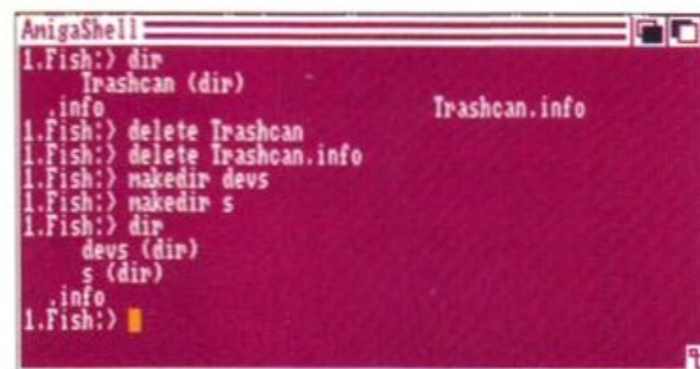
Using the CLI, it's easy to create the two drawers that must be on every self-booting disk.
