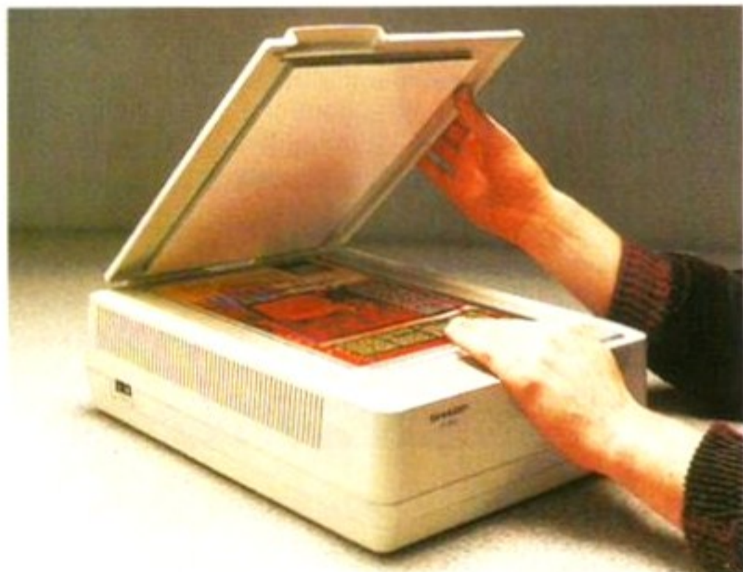
The Sharp JX300 is a true flat bed scanner, and requires both a pokey Amiga and a fairly expensive interface board.
