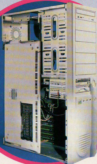
The Eyetech Tower uses a specially modified case which allows an A1200 to be fitted easily and securely. This is definitely one of the easiest solutions to building your own computer.
