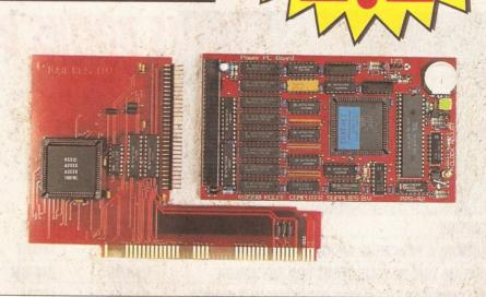
The KCS emulator is available as a trapdoor expansion for the A500 and A500 Plus, or as a plug-in card for the A1500/A2000/A300 series. It comes with 1Mb of extra memory, too
