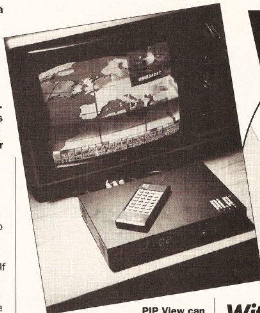
PIP View can show two video signals on the same screen at the same time – all under remote control
