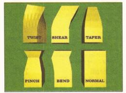
A new set of modelling tools provide several kinds of deformation. How the object is affected depends on the type of deformation and where the object's axis is located. or extruded) objects. Note the lens flares and global haze effects in the rendered image. These too are new features, but I've seen better in other software.
