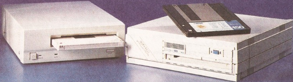
On the left we have the MoMiga Magneto-Optical Drive, while on the right we have the Bernoulli Box.
