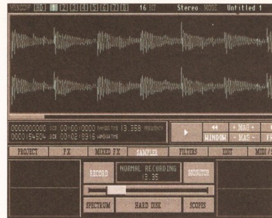
The two windows at the bottom display the incoming sound waves. The recorded sample is displayed in the main window above.
