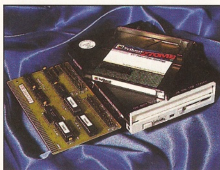
An internal SyQuest IDE drive. It requires an IDE controller like the Tandem pictured here.
