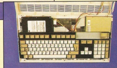
Step 6: The drive should fit snugly, and you can now replace the lid and re-attach the power.
