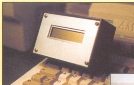
Above: The prototype LCD built as an external unit for non-boxed Amigas.
