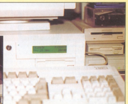
Above: The completed Liquid Crystal Display (LCD) in place in my A4000.
