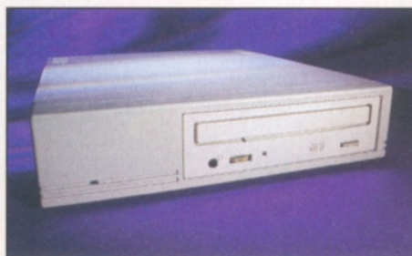
IDE drives are much cheaper than SCSI and you can now have up to four on one A1200.
