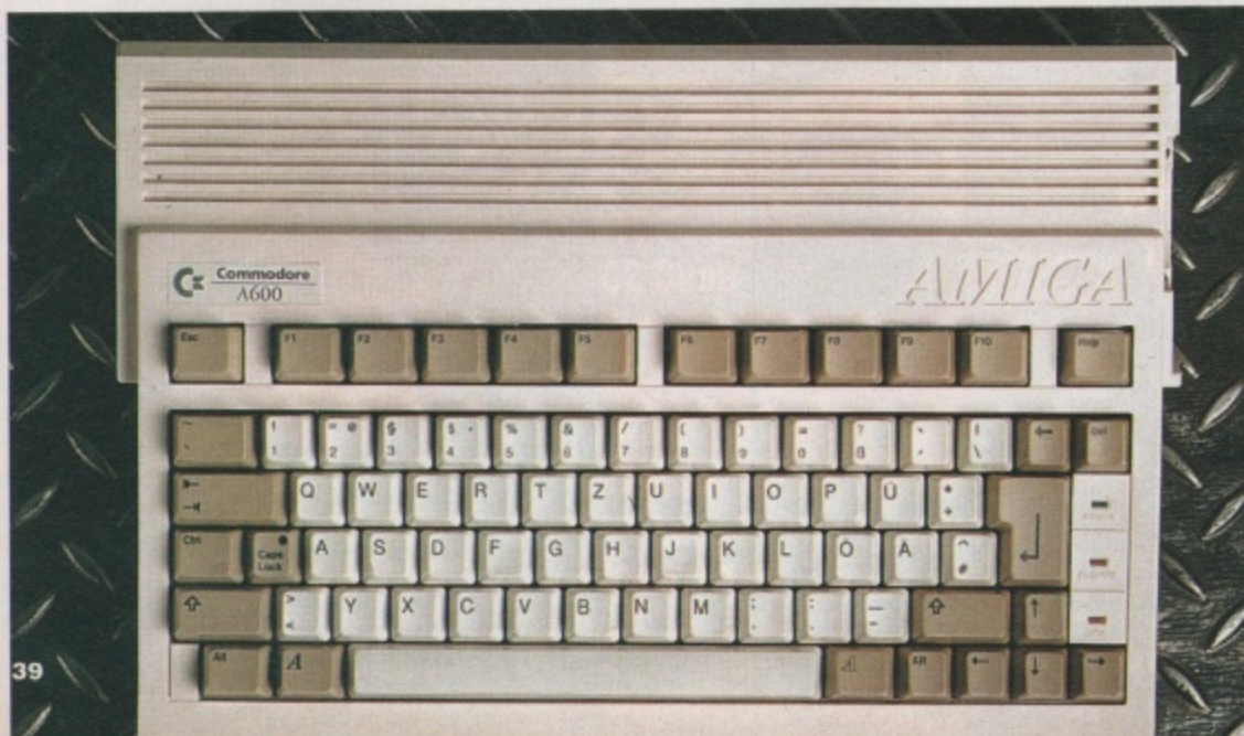
As with the A570, surface mount technology makes for a more compact design. All the original connectors of the A500 have been retained, with the exception of the Mono Video Out port, which has evolved into Composite Colour. The modulator is internal now, too.
