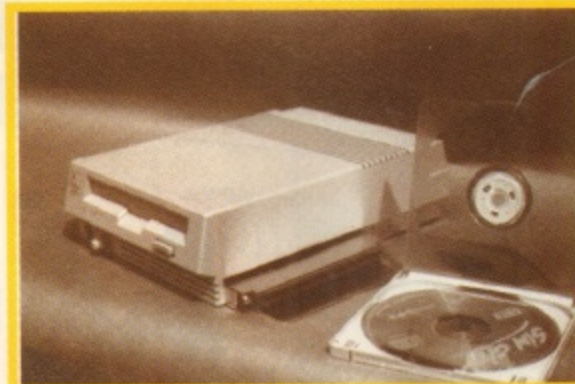
▲ No not a CD1200, but an A570. Commodore's first CD-ROM drive. Compatible with the A500s the A570 gave Amiga owners access to mass storage at a low price.
