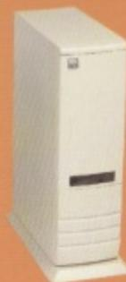
The tower comes complete with 6 x 5.25" drive bays, 5 x 3.5" drive bays, 7 x Zorro slots, 5 x PC slots, real time clock and a 230 watt power supply.
