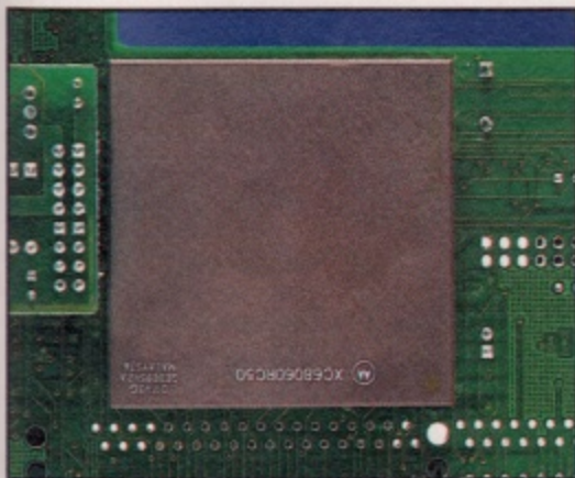
▲ The 060 chip is actually cooler than the 040, hence no fan.
