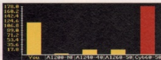
▲ A telling examination of how the 040 and 060 CPUs perform emulating the complex FPU instructions used in ray tracing.
