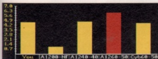
▲ In a test of raw memory speed, the Apollo 1260 shows it has the fastest memory interface on the Amiga.
