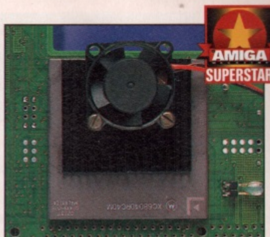
▲ The 1240 needs both a heat sink and a fan to keep cool.
