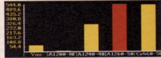
▲ Using basic FPU instructions which are in the 040 and 060, the flops benchmark shows the 060s performing very well.
