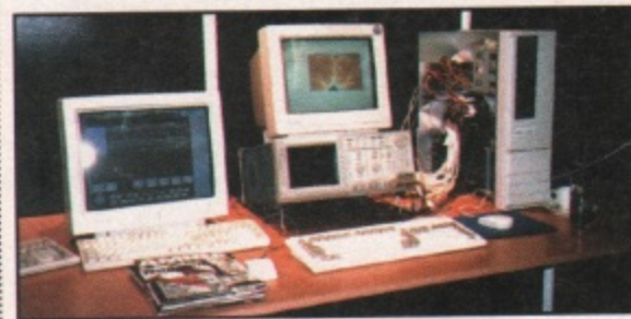
Shown here is Phase 5's development system for the Power Up project. The unit under the middle monitor is a logic analyser connected via a bundle of wires to the 200MHz PPC604 inside the 4000 Tower.
