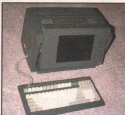
▲ QuikPak's A4060L 'luggable' video editing system based on an Amiga and a NewTek VideoToaster.
