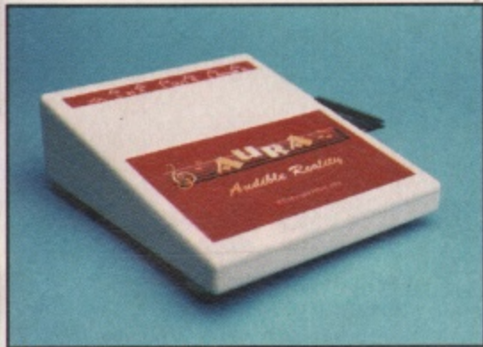
▲ With the new mixing and disk recording options you can now take more advantage of Aura's single channel 16-bit output.
