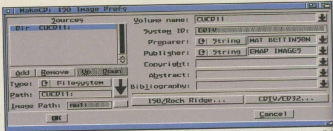
▲ The source preference for the data track in MakeCD. Setting the source of the files to build and the so-called 'Primary Volume Descriptor' where things like the preparer and publisher and the volume name are set.
