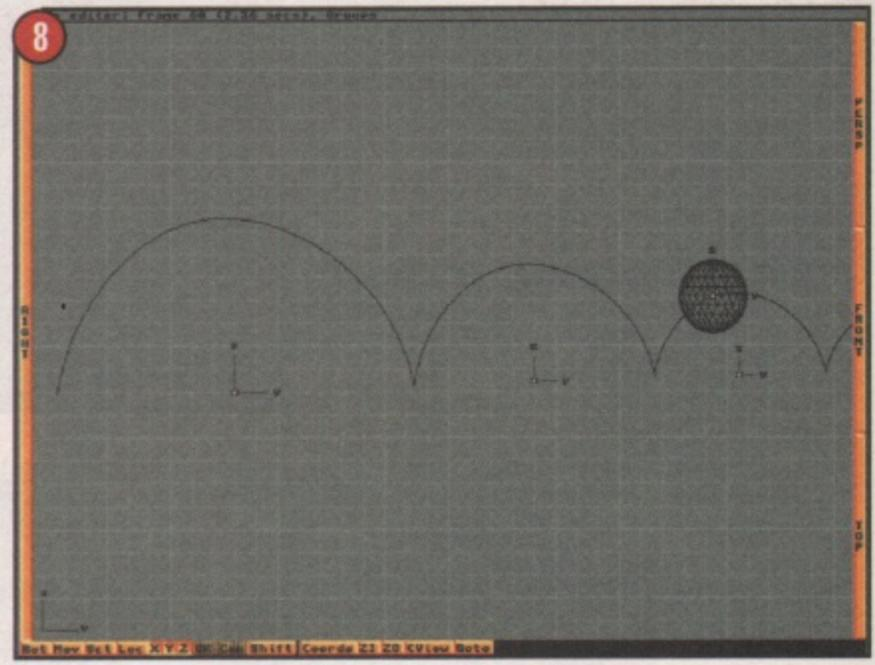
this isn't the path we want. So select the end points, and rotate them in the X axis. The curve will change shape and you'll be left with this arc. This looks pretty much like the path which a bouncing ball would take. Make sure you save it. See pic 3.
