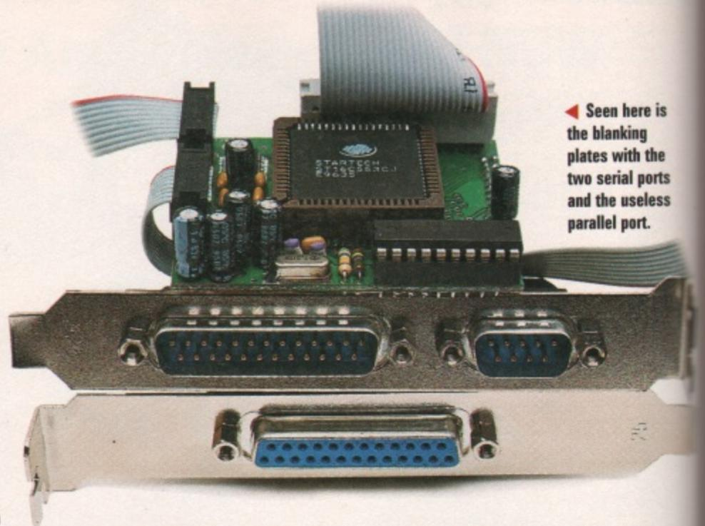
◀ Seen here is the blanking plates with the two serial ports and the useless parallel port.
