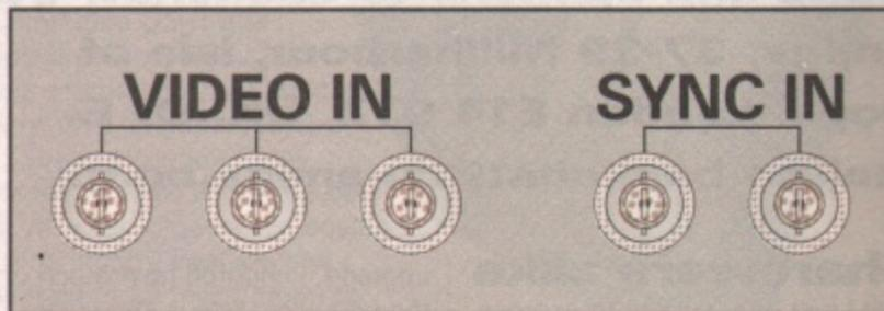
then you have a BNC type. VGA BNC adapters can be bought from Maplin (tel: 01702 554000) for just under £20. These will terminate into a 15 way, high density D type connector - the standard for PC monitors. You will need to get an Amiga monitor adapter too - many of our advertisers sell them, try First Computer Centre (tel: 0113 231944) for example.
