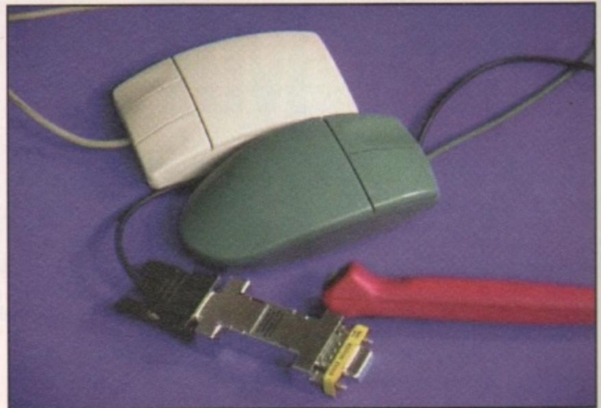
▲ The Topolino allows PC serial input devices such as mice, trackballs, or even infra red controls to work on your Amiga. It just sits between the mouse port and the serial device.
