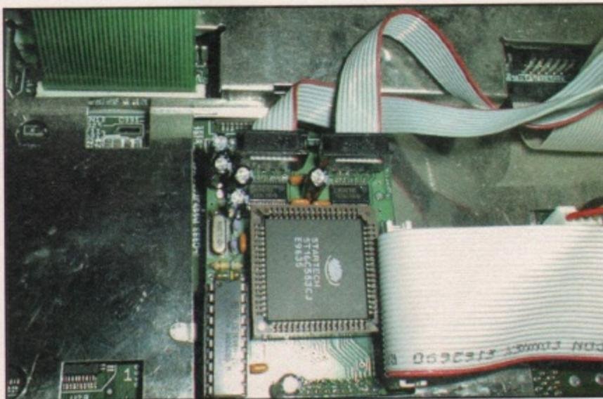
▲ This shows the PortPlus dropped into the hole that's revealed after the hatch in the RF shield is removed. It's designed to perfectly fit the hole and plug onto the clock connector.
