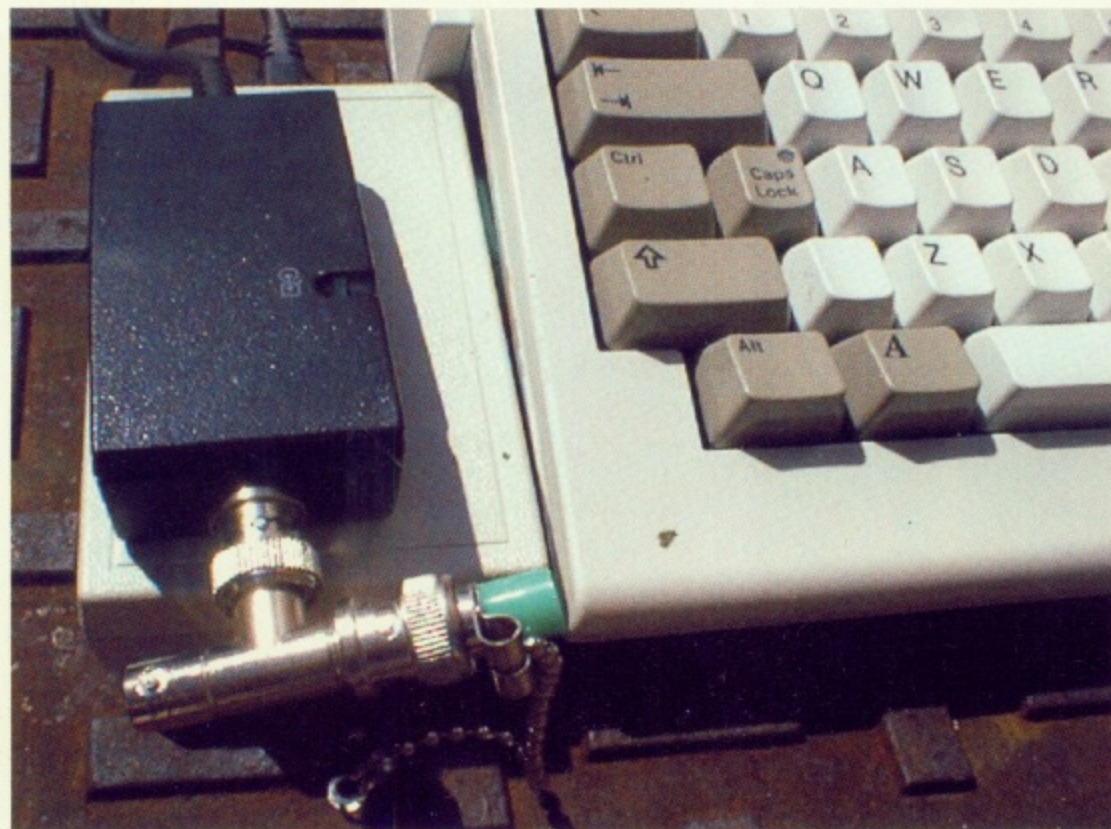
► Here's the A1200 Ethernet prototype showing the main interface and the BNC adapter.
